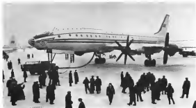
Tu-114, with one engine being overhauled, is parked next to An-12 Embler at a Krasnoyarsk airport. Tail of the An 12, a four-engine turboprop designed for Aeroflot's rough field landing operations, shows obvious cutbacks in an endeavor to solve a structural stability problem. Heavy truck under nose of Tu 114 is typical of ground loading equipment at Krasnoyarsk airport.
